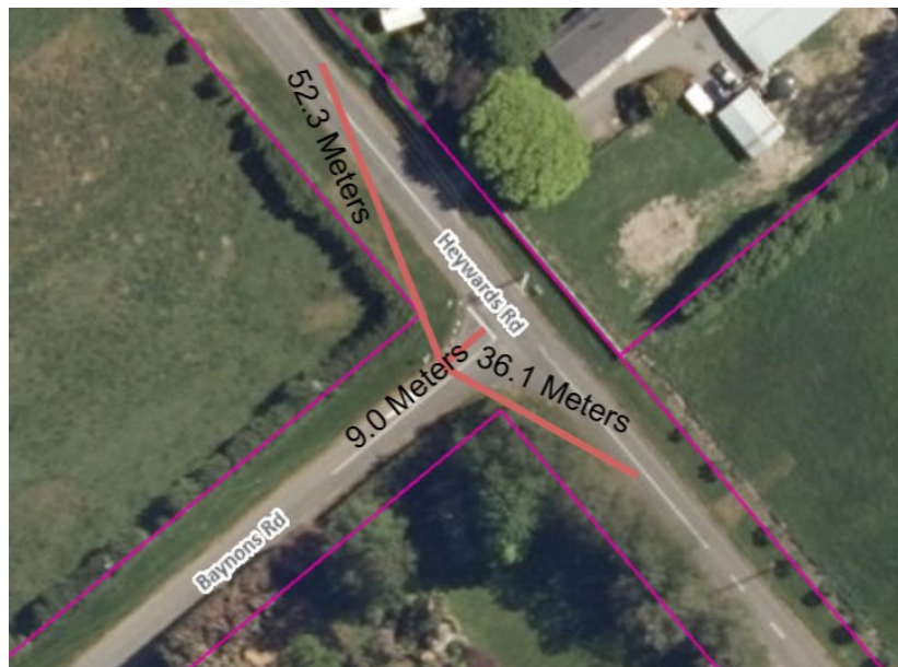
Figure 2: Available Sightlines at Baynons Road / Heywards Road intersection
