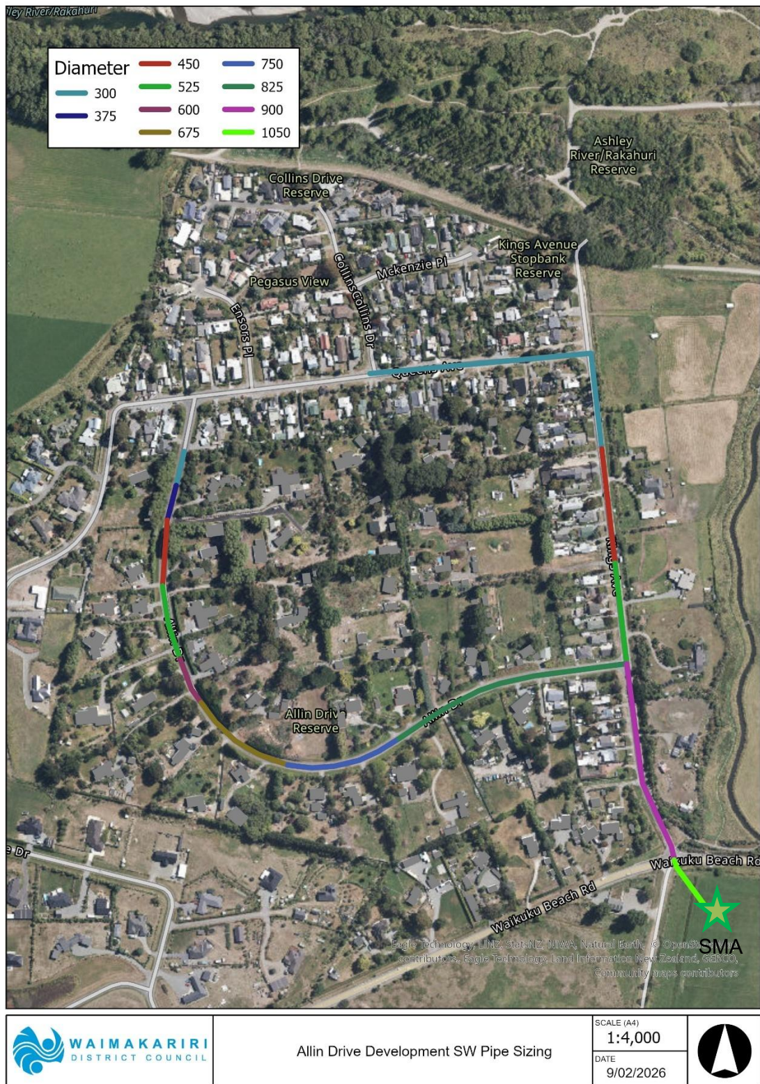
Figure 7: Stormwater Pipe Sizing
