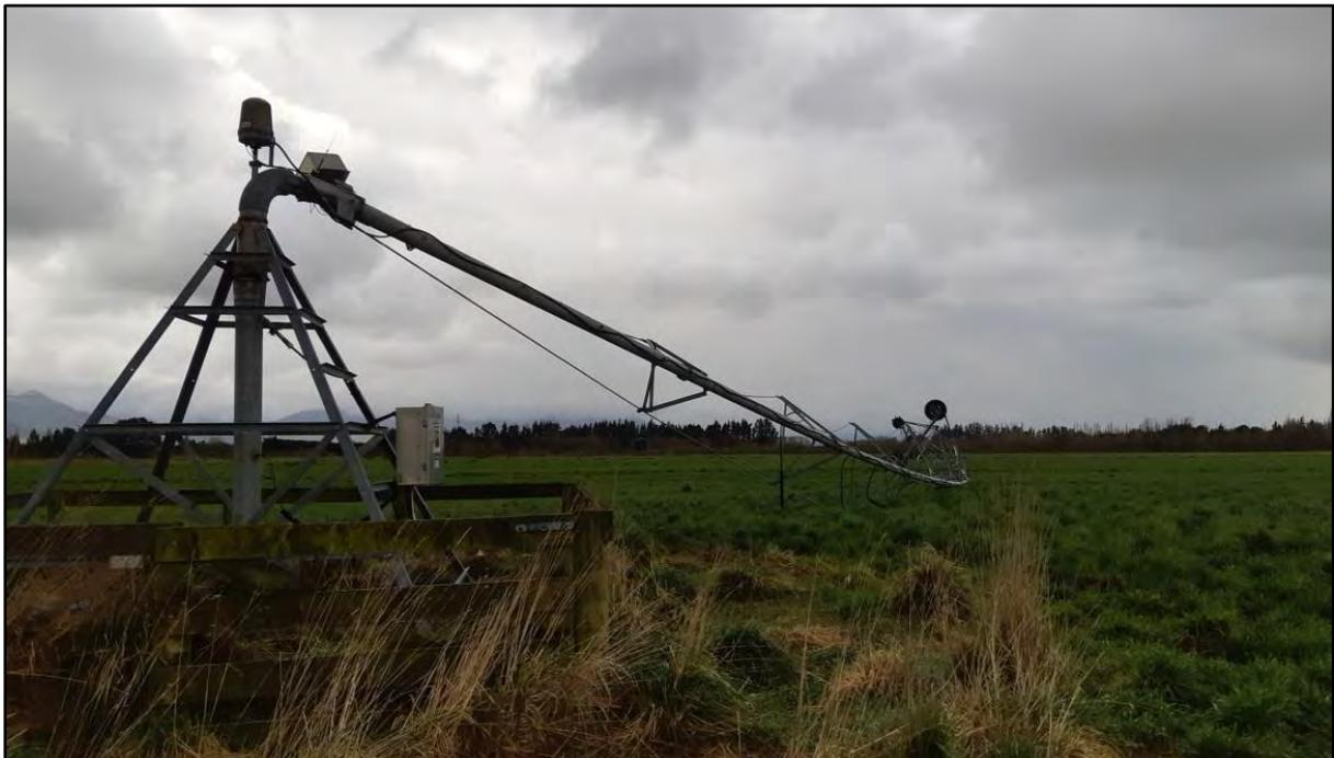
Figure 9. Damage to the western irrigator during the September 2021 wind event
