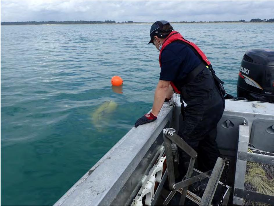
**Figure 3-2:** Deploying the drifting drogue for water quality sample collection.
