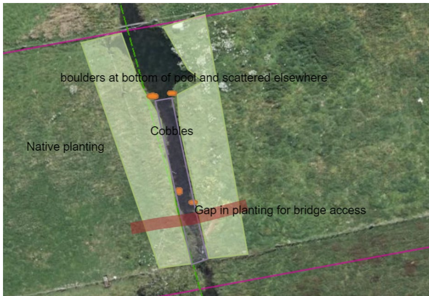
Figure 4: Restoration at 428 Tuahiwi Road. The light green indicates native planting that is proposed to be carried out. Boulders and cobbles have been added to improve in-stream habitat.
