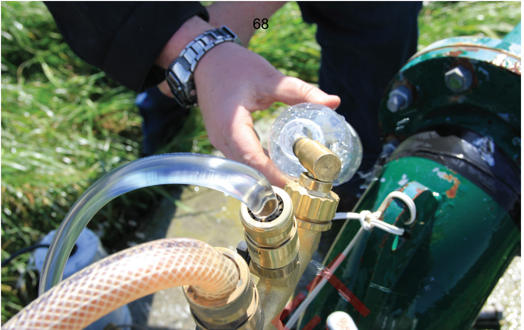
Taking a water sample at a wellhead
