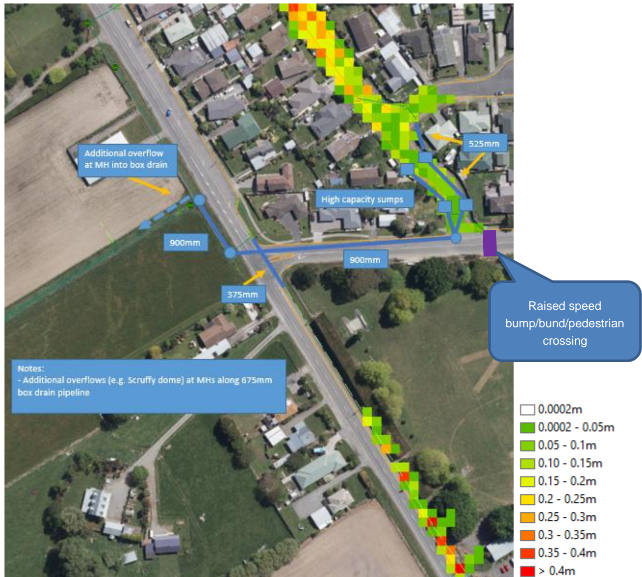
Figure 5 Predicted flood depth for the refined concept option during a 1 in 50 year 2 hour critical duration storm event
