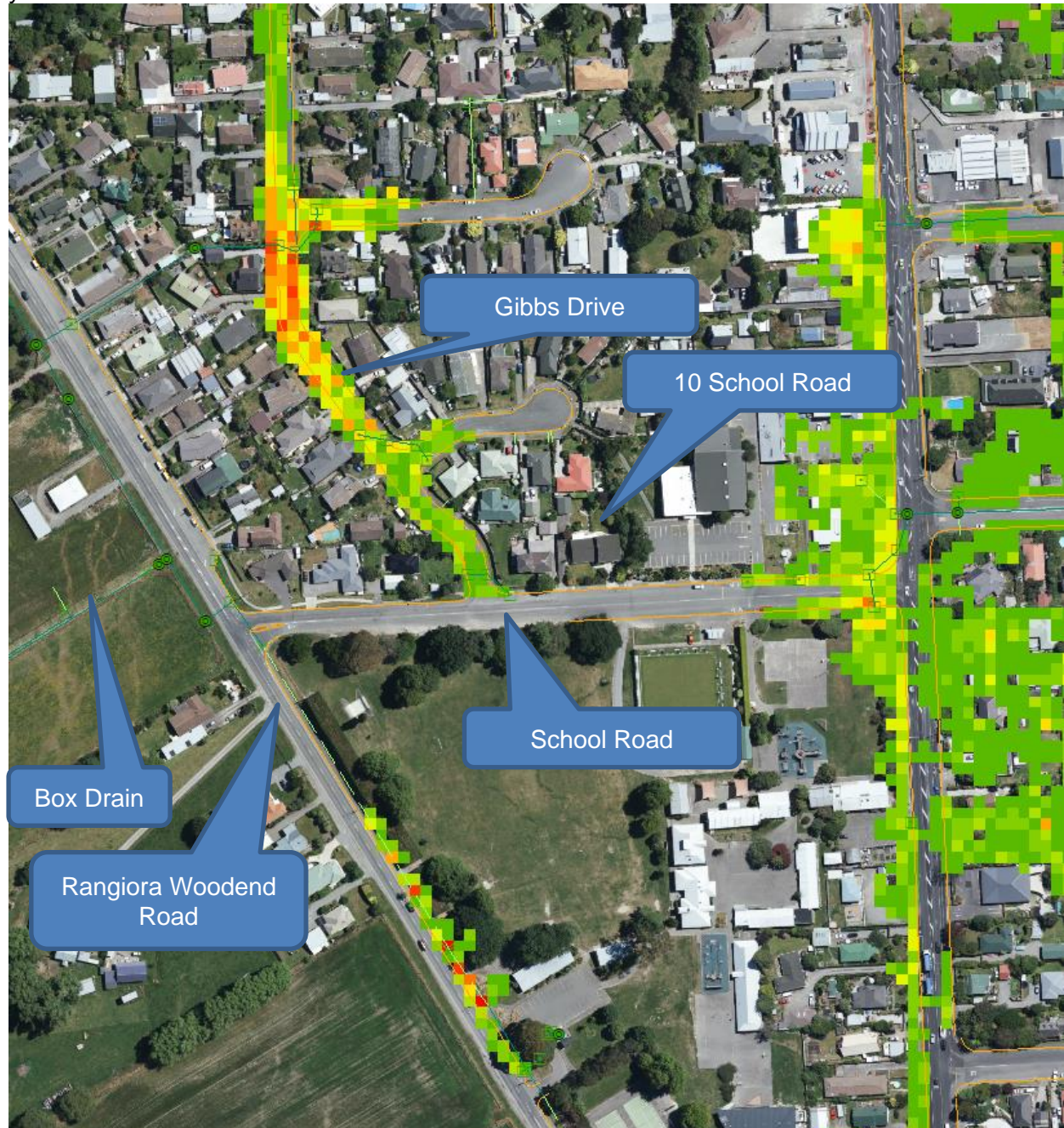
Figure 7 Predicted flood depth within wider catchment for the refined concept option during a 1 in 50 year 2 hour critical duration storm event
