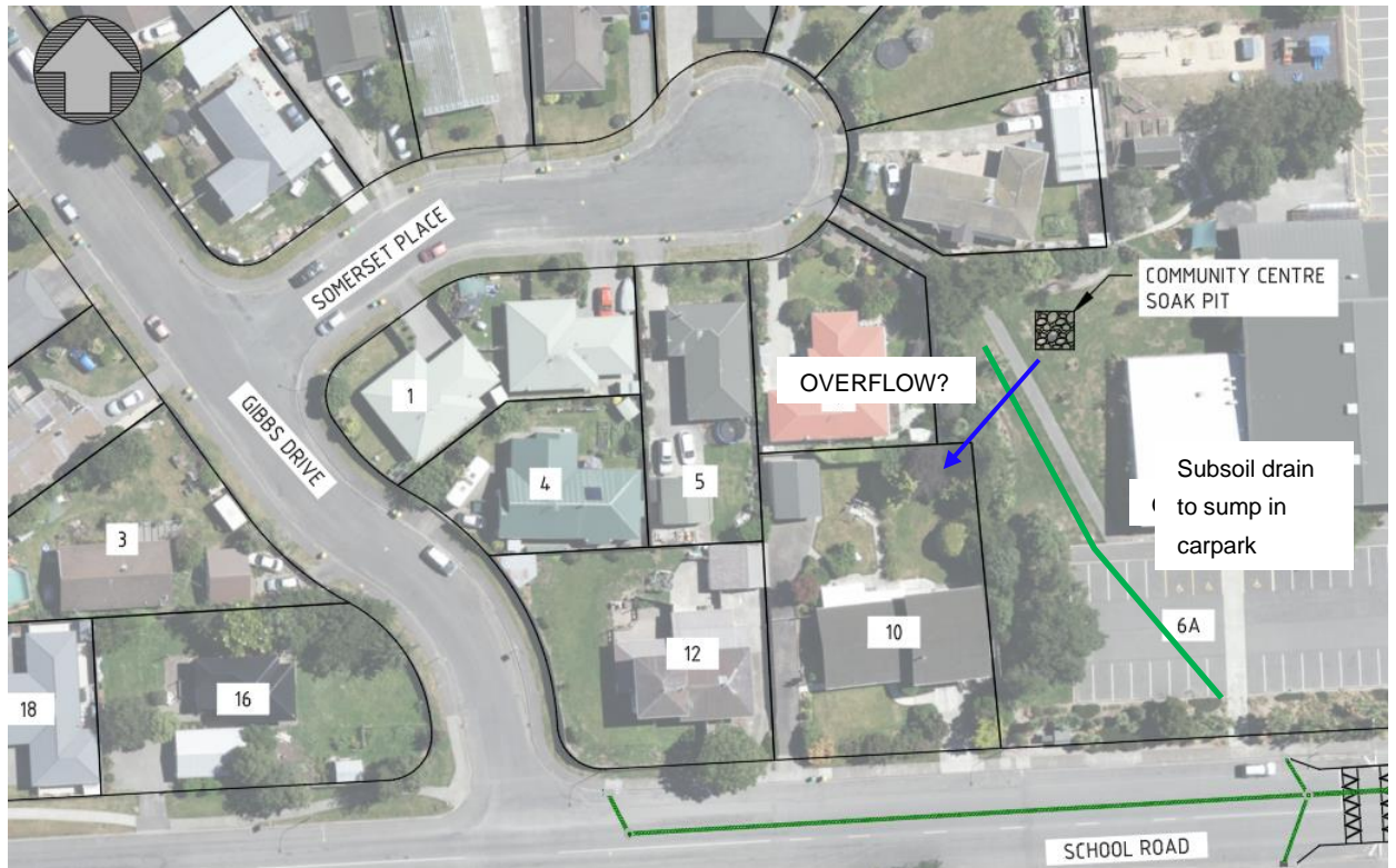
Figure 11: Community Centre Soak Pit
