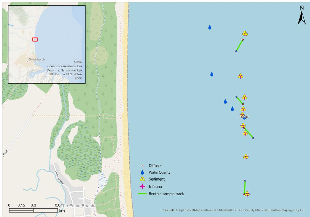
**Figure 3-1:** Map showing location of the outfall diffuser relative to the city of Christchurch and Pines Beach. Locations of sediment grabs for chemical analysis and infauna counts, water quality samples and benthic sampling tows are also included.
