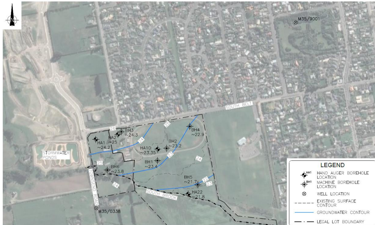
Figure 4: Preliminary Median Groundwater Contours from Site Observations
