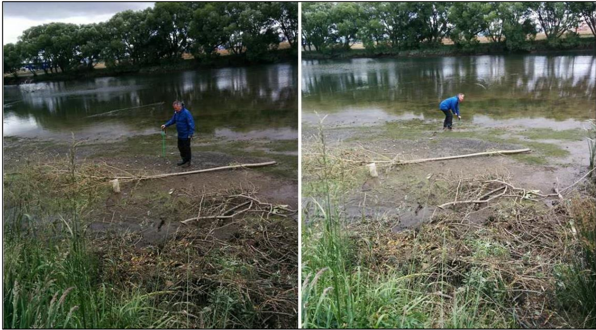
Figure 3.5 The right bank edge of the sediment trap is a firm sandy-silt-gravel mix with an abrupt change to fine sediment
