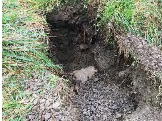
Photo 7: Detail of Test Pit 1 - note groundwater at the base of the pit and collapsing side walls
