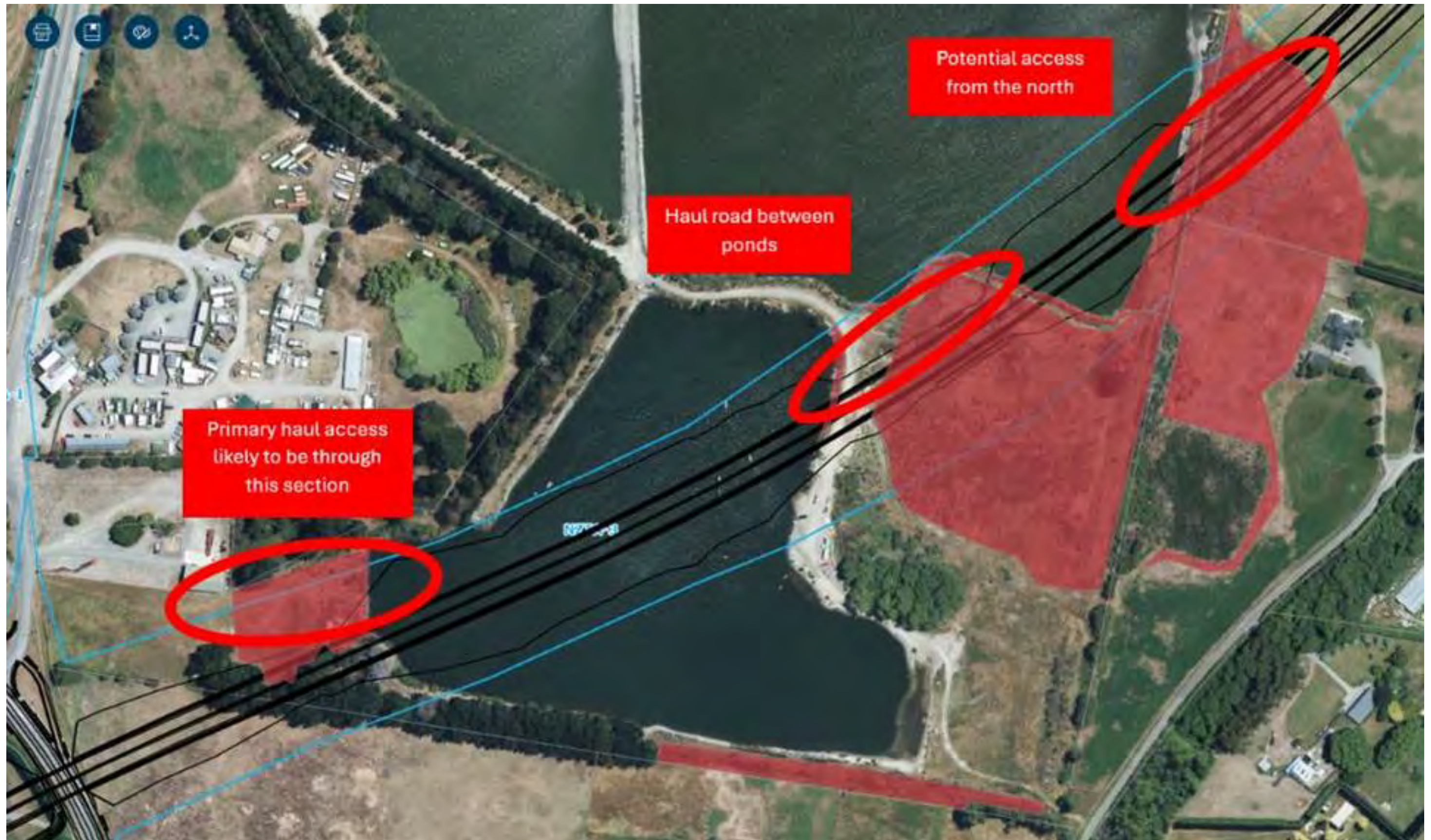
Figure 12 – Proposed indicative early works development footprint within the Ready Mix Concrete area. Blue lines indicate the development footprint. Red areas indicate lizard habitat. Red circles indicate the likely areas where development will be undertaken. However, these are subject to change.
