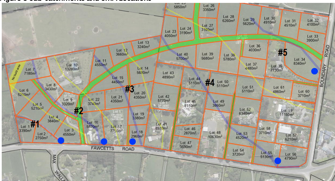
Figure 5 Sub-catchments and SMA Locations
