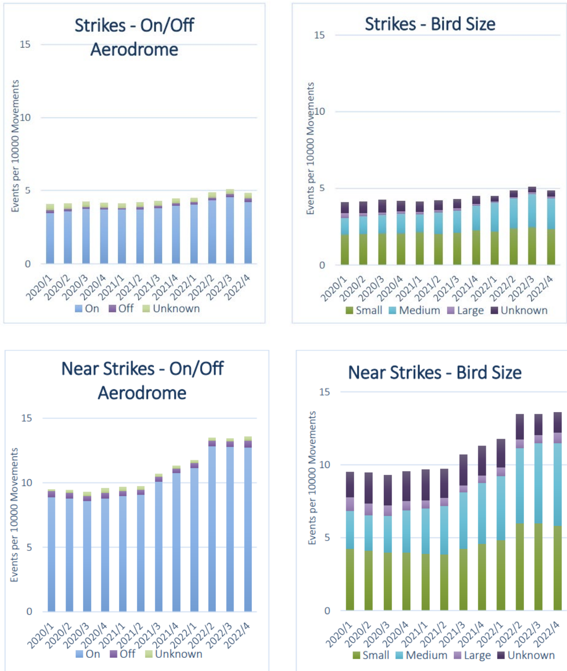
Figure 2: Bird strike rates per 10,000 aircraft movements at all New Zealand aerodromes (12-month moving averages) – strikes and near strikes (taken from CAA 2023).
