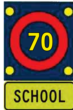
70km/h variable speed limit school sign for roads with a 100km/h permanent speed limit
