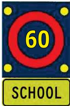
60km/h variable speed limit school sign for roads with an 80km/h permanent speed limit
