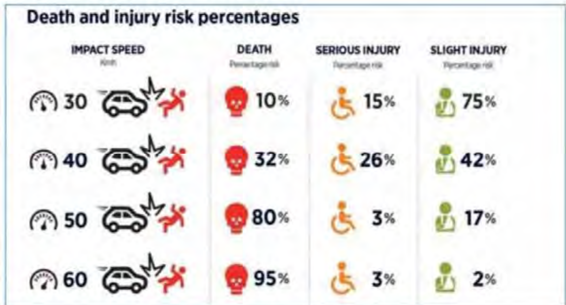
Figure 1. Death and injury risk percentages for pedestrians at different vehicle speeds (Auckland Transport).
