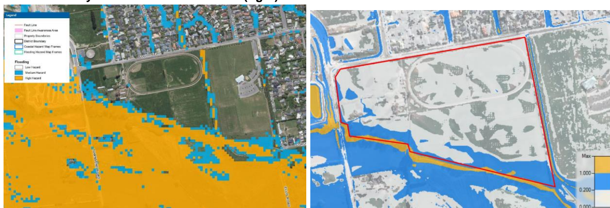
Figure 10 and Figure 11: Comparison of WDC hazard map (left) and RILEY flood assessment modelling results of 200-year combined flood event (right)
