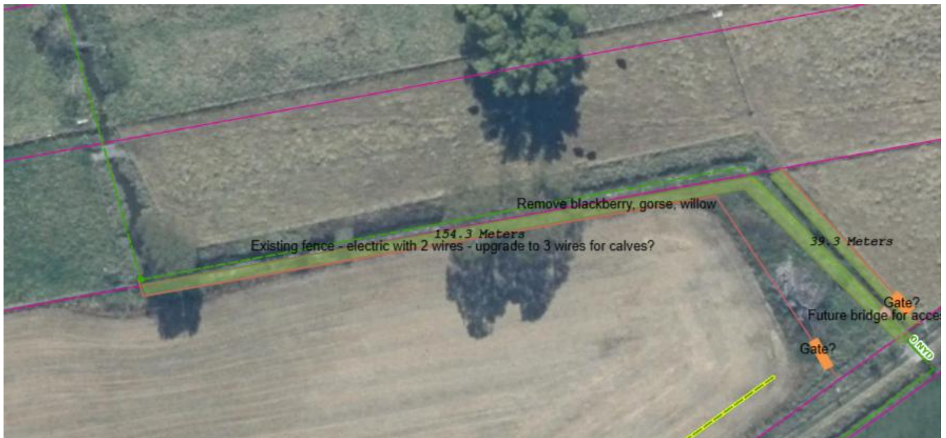
Figure 1: Tuahiwi Road property. Pink indicates property lines. Green indicates the areas for planting, dotted green line shows the waterway location, orange indicates the location of the new fencing with a least a 3m setback from the waterway.
