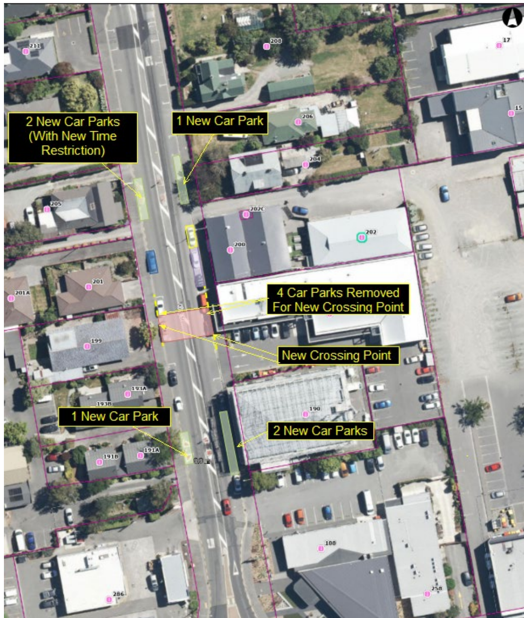
Figure 2: Proposed location for new refuge Island and re arrangement of on-street car parks.
