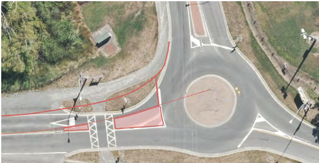
Figure 1: West approach realignment (retaining south kerb)
