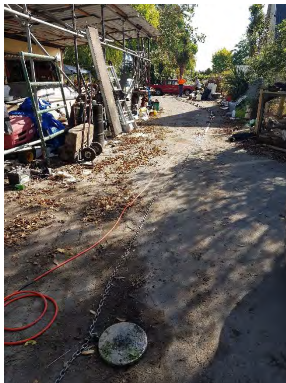
Geophone array and aluminium plate set up on Line 5.
