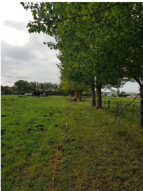
MASW survey along fence line for Line 3.
