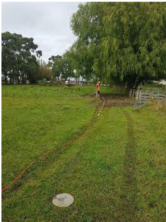
Geophone array and aluminium plate set up on Line 1.
