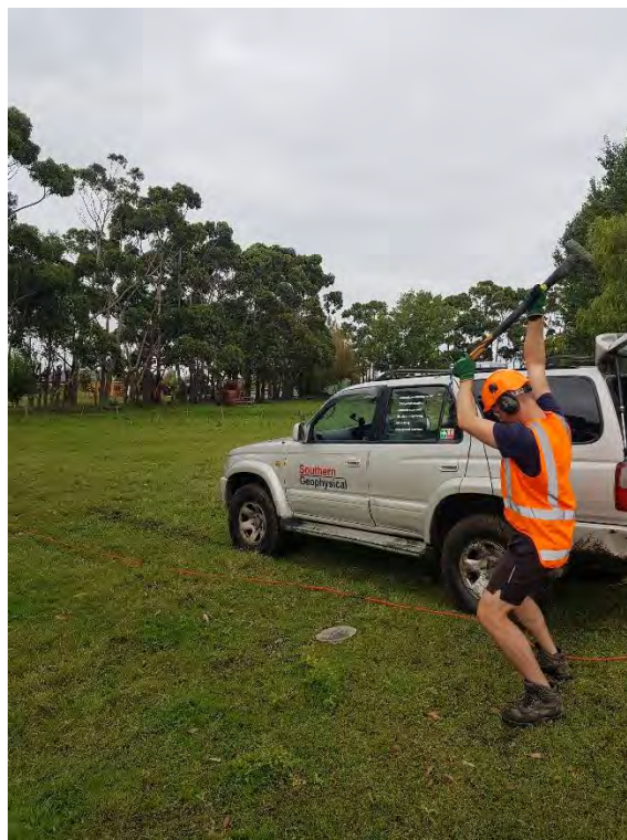
MASW data acquisition on Line 2.
