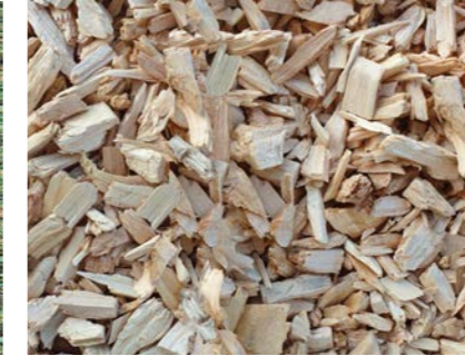
PLAYGROUND SOFTFALL Woodchip safety surfacing
