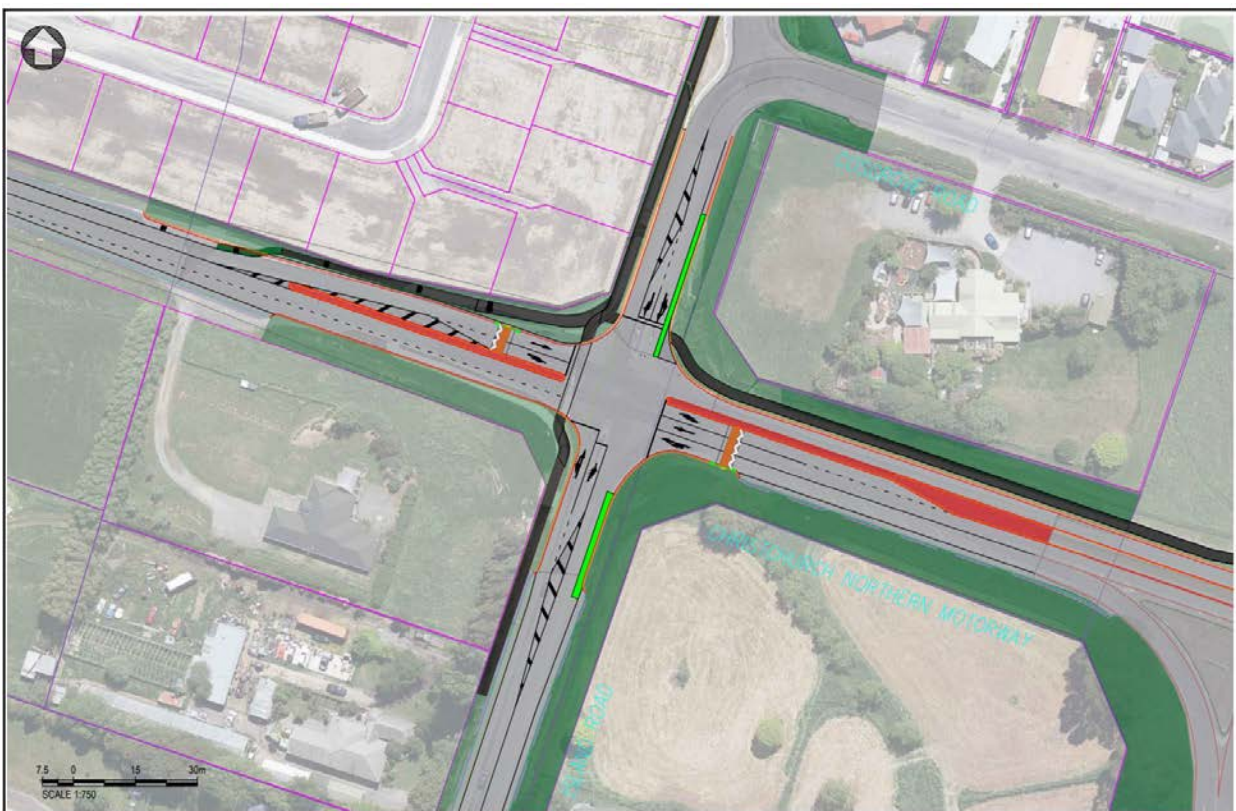
Figure 14 Traffic signals option scheme design (WDC design)
