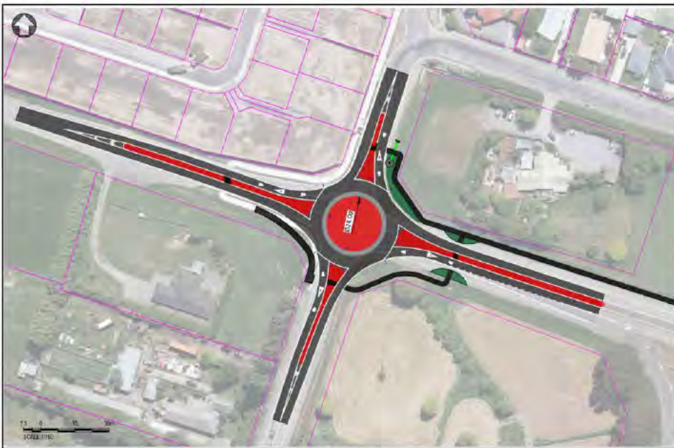
Figure 16 Single-lane roundabout option scheme design (WDC Design)
