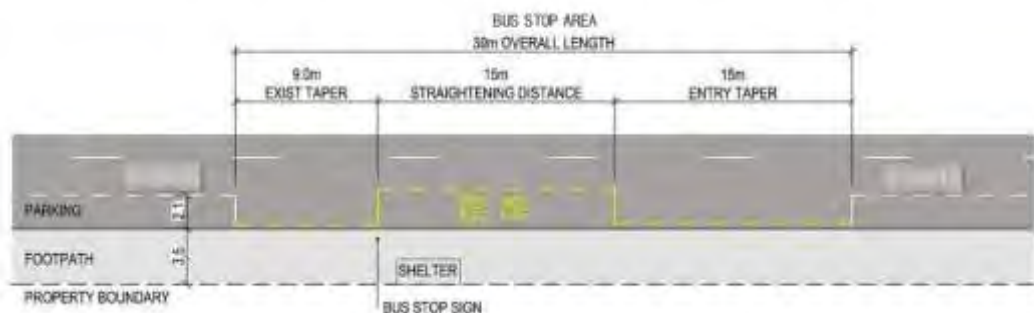
Figure Three: Waka Kotahi minimum bus stop dimensions
