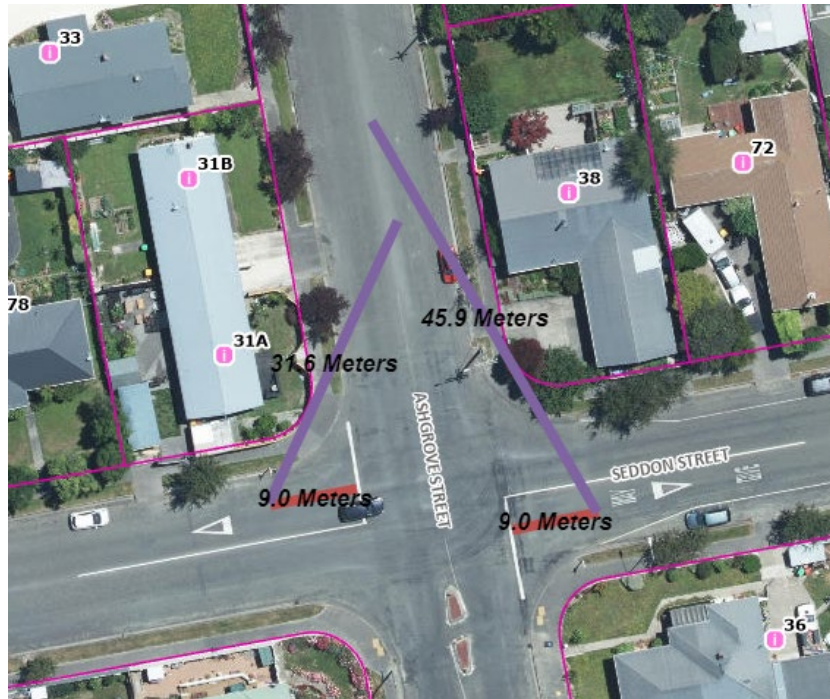
Figure 4. Available sight distance at the intersection of Seddon St and Ashgrove St
