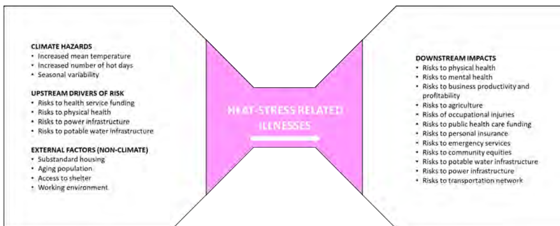
Figure 20.14: Bow tie diagram illustrating the causes and effects of risks to heat-stress related illnesses.
