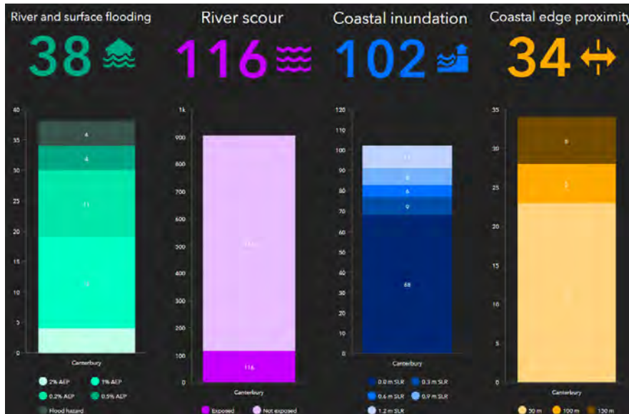
Figure 11.4: Exposure of landfills in Canterbury to flooding, scour and coastal inundation (Tonkin & Taylor, 2020).
