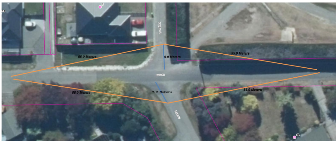
Figure 7: Sightlines as per TCD Manual at Vaughan Street / Buller Street / Cross Street intersection.
