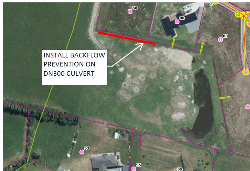
Figure 13 - Culvert back-flow prevention install
