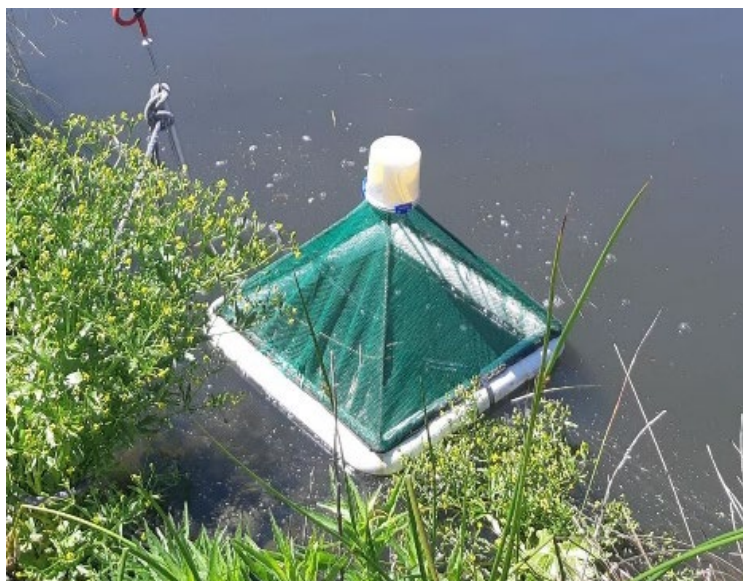
Figure 3. Aquatic Fly Emergence Trap. Note that the design has been modified slightly to make the traps more suitable for a wastewater environment
