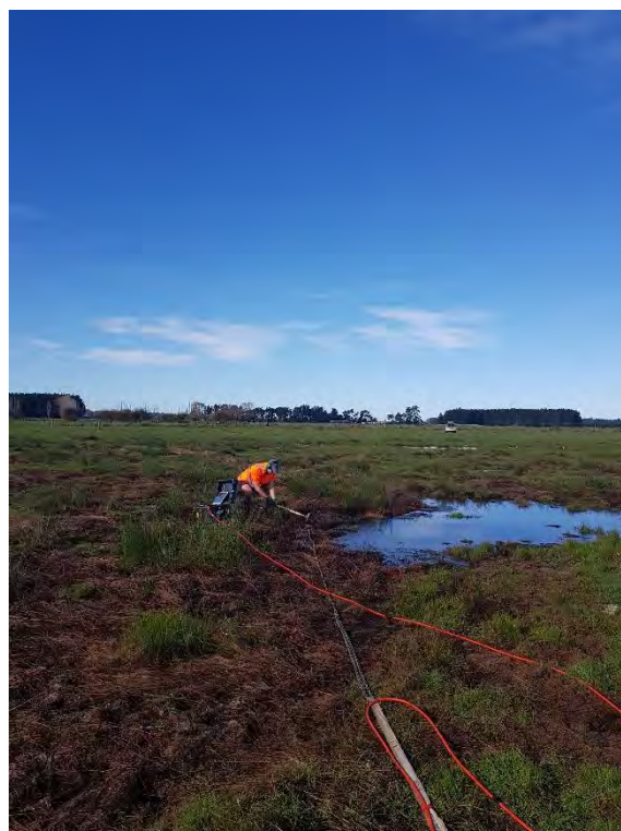
MASW data acquisition during swampy hand-towed section of Line 4.
