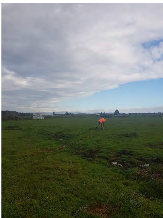
GPS acquisition on northern end of Line 6. MASW line passing over small saturated surface depression.
