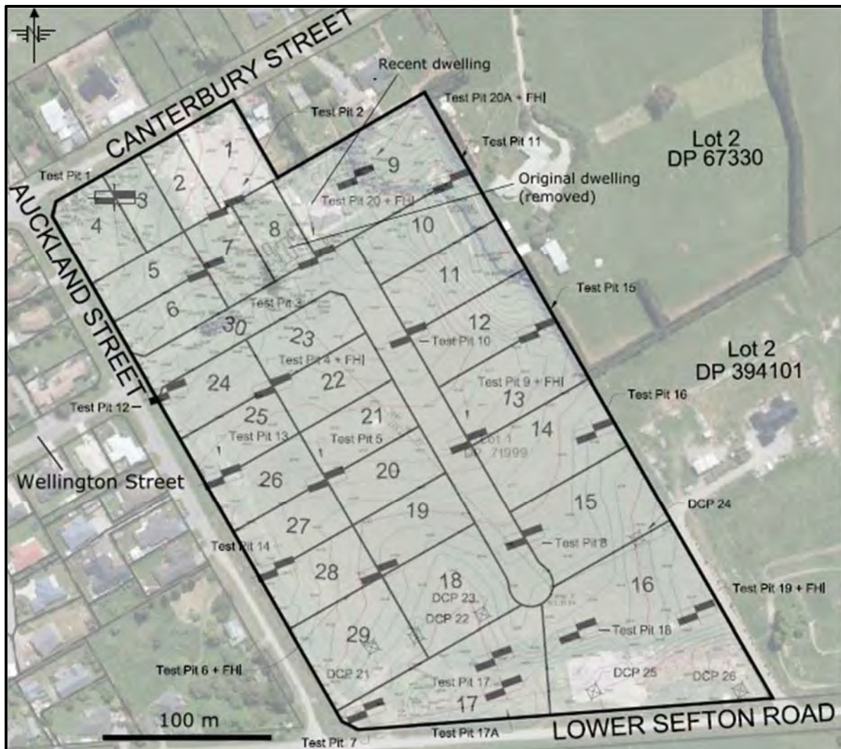
Figure 3: Proposed scheme plan (dated 09/20) showing test pit locations, a recent aerial image 5 and an overlay of existing topographical contour plan 2 . Contour intervals are 0.2 m (blue) and 1.0 m (red). Note that the existing “original dwelling” marked on the topographical contour plan in the area of proposed Lot 8 was removed prior to this investigation.
