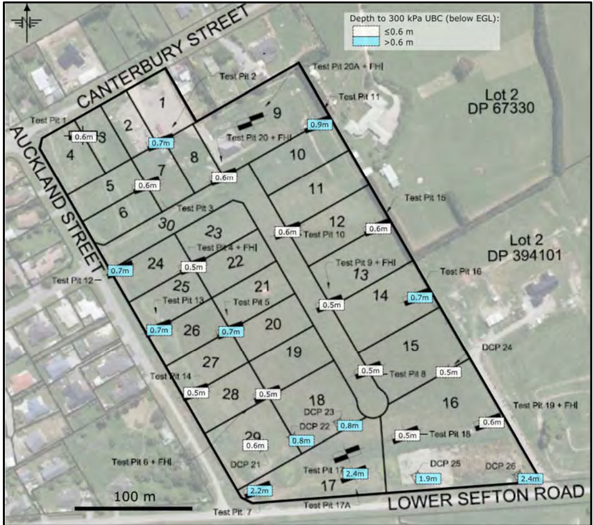
Figure 10: Map of the proposed development showing the depth 300 kPa (UBC) below EGL encountered across the site.
