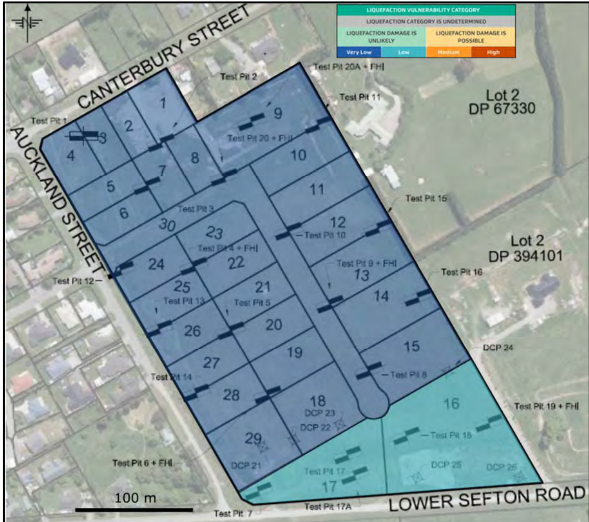
Figure 9: Expected liquefaction vulnerability categories at the site based on subsurface observations. Category extents defined by proposed lot boundaries. Categories based on MBIE (2017) 22 .
