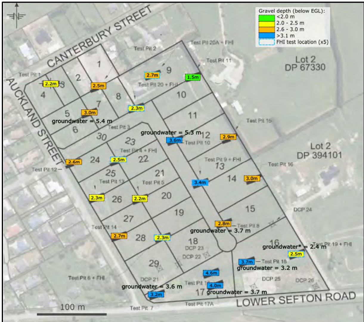
Figure 8: Proposed scheme plan annotated to show the approximate depth to gravel and groundwater (m below EGL) measured in test pit excavations during the site investigation.
