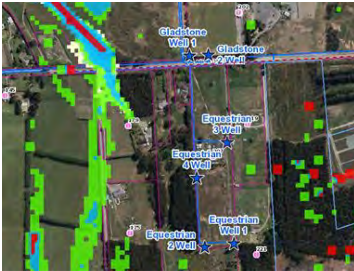
Figure 3: Flood Modelling for EQ and Gladstone Wells (coloured squares indicates flood zones).
