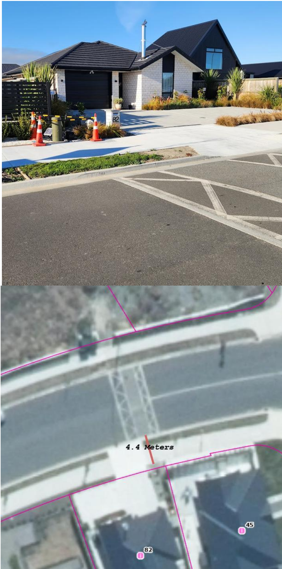
Figure 3 - 82 Silverstream Blvd – monitoring location (note: 4.4m measurement is taken from fender to hexanode as measured on site)
