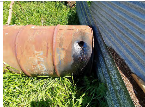
56: Oil drum lying on its side which has been pierced and is leaking oil.
