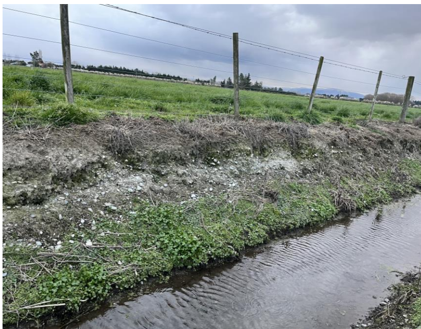
Figure 6: A drain near the north of the Site shows loamy textures Gley Soil over gravels
