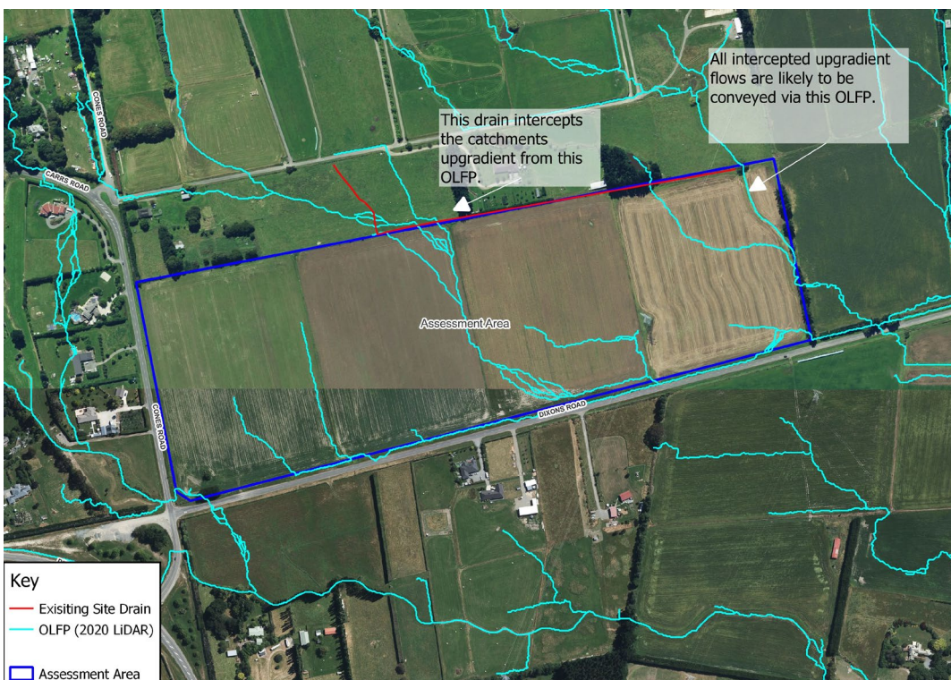
Figure 2: Overland Flow Paths generated using the 2020 LiDAR.
