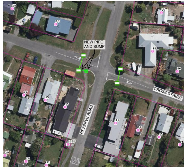
Figure 3. New sump and pipe recently installed by Roding at the intersection of Cross Street and Reserve Road.
