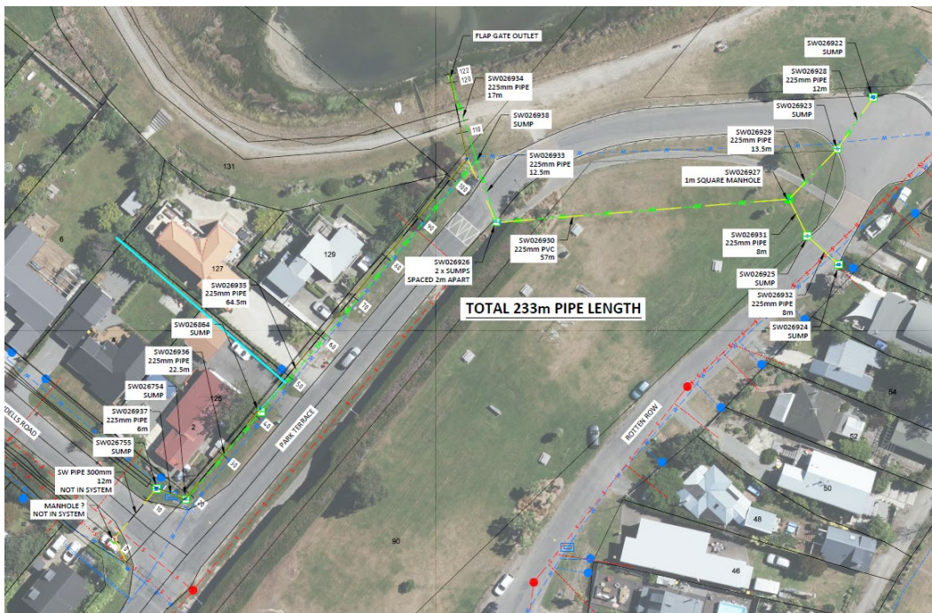
Figure 3 – Pipework CCTV inspected in the Swindells Road / Park Terrace area
