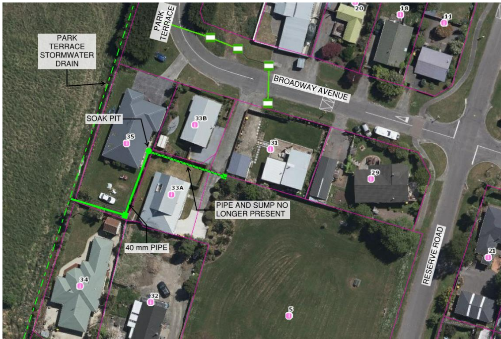
Figure 4. 35 Broadway Avenue stormwater pipes.
