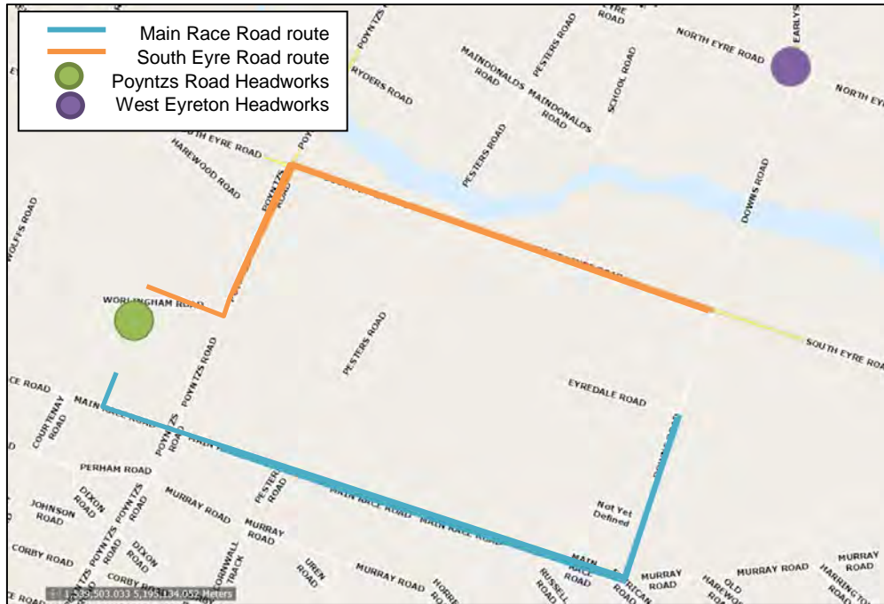
Figure 1: Potential Pipe Routes for Connection of Poyntzs Road to West Eyreton (exact point at which schemes will join is subject to hydraulic modelling being finalised)
