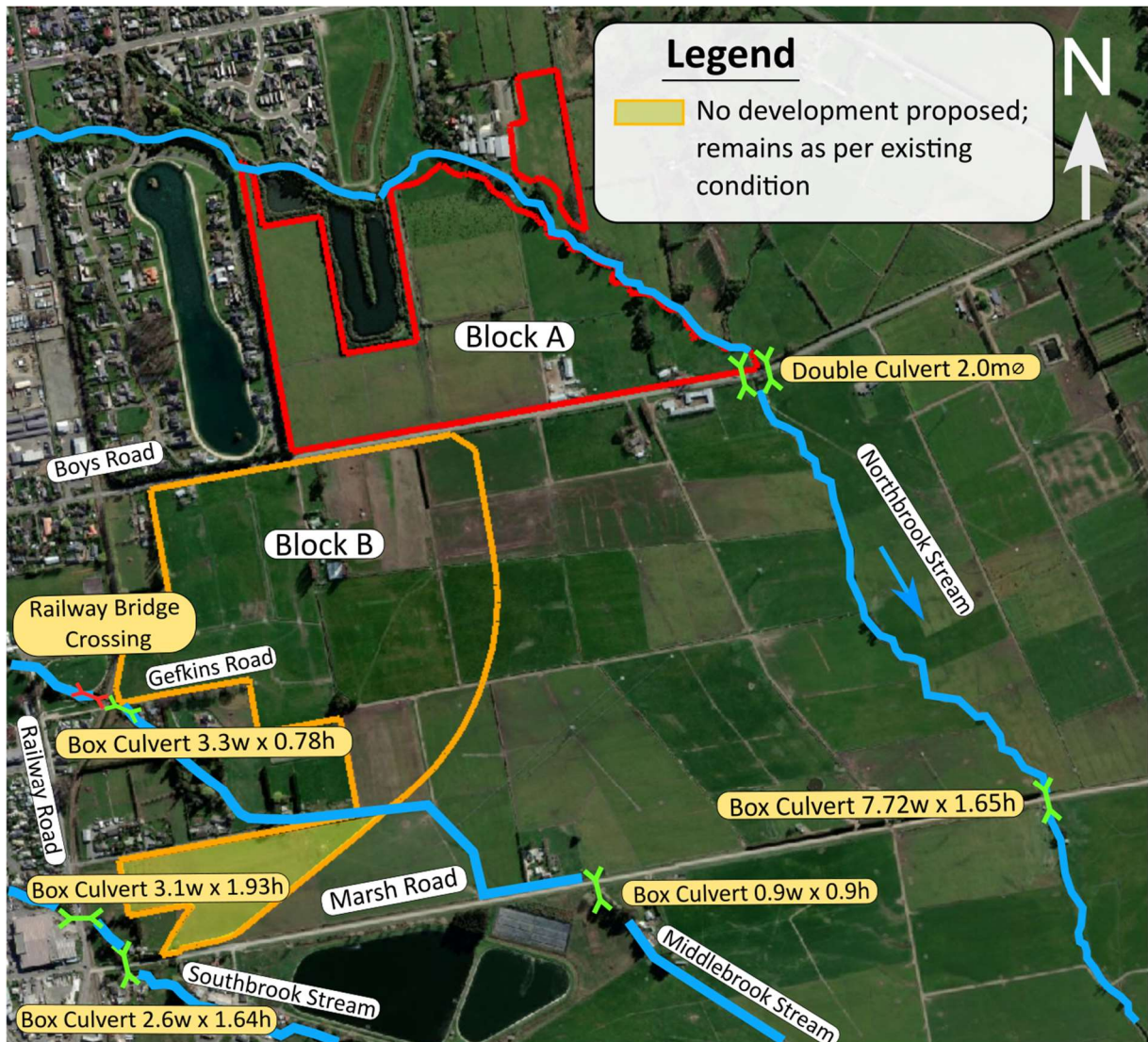
Figure 1: Block Delineation, with blue showing streams and green showing culverts
