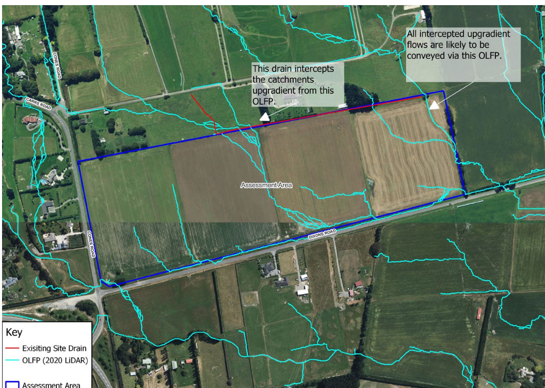
Figure 2: Overland Flow Paths generated using the 2020 LiDAR.
