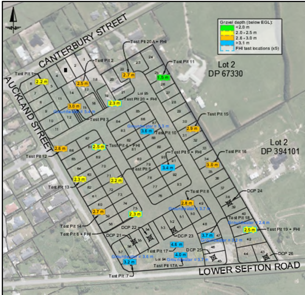
Figure 8: Proposed scheme plan annotated to show the approximate depth to gravel and groundwater (m below EGL) measured in test pit excavations during the site investigation.
