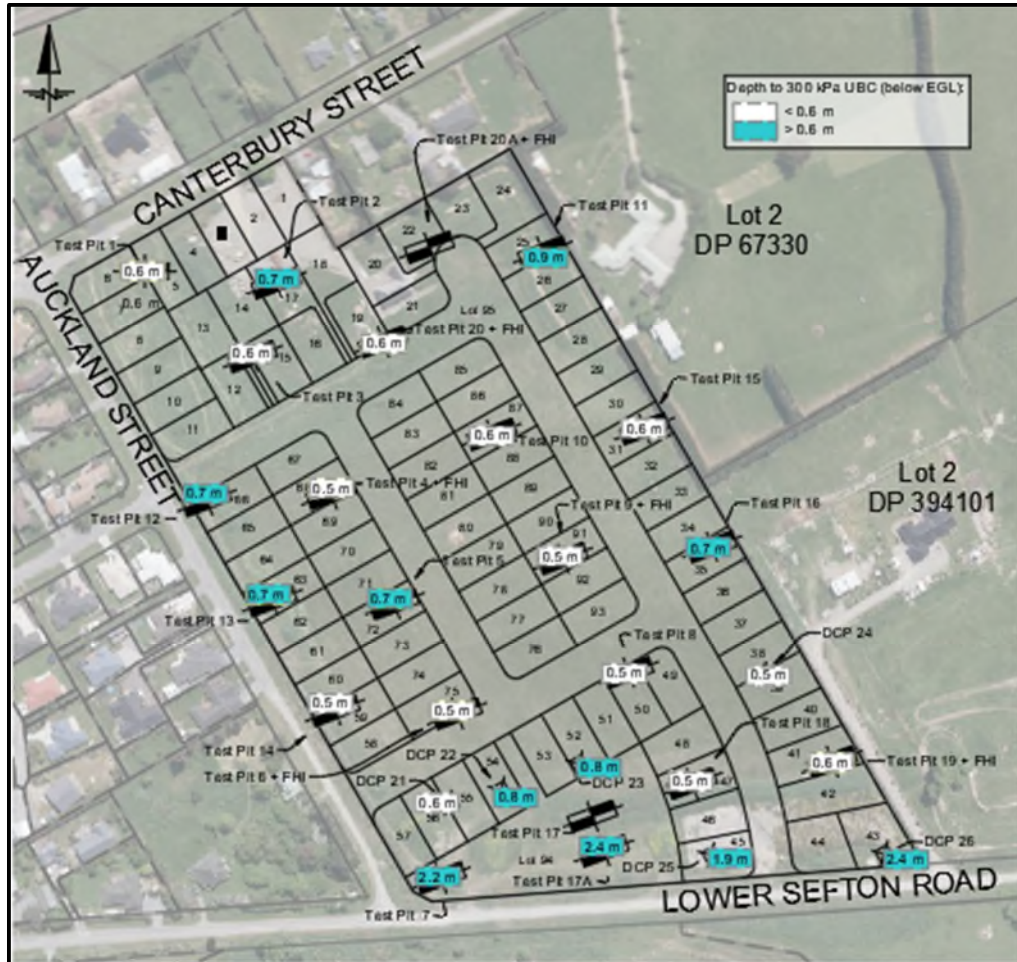
Figure 10: Map of the proposed development showing the depth 300 kPa (UBC) below EGL encountered across the site.
