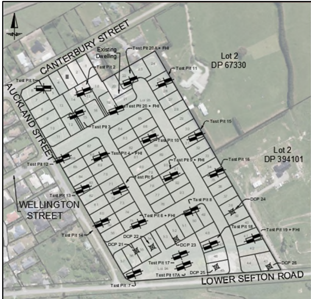
Figure 3: Proposed scheme plan showing test pit and DCP locations and recent aerial image 5
