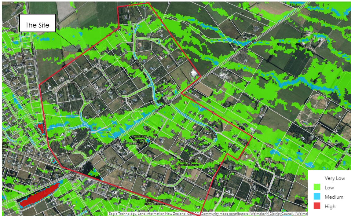
Figure 4. 1 in 200 year Flood Hazard map for the Site (Source: Waimakariri District Flooding Hazard Maps)
