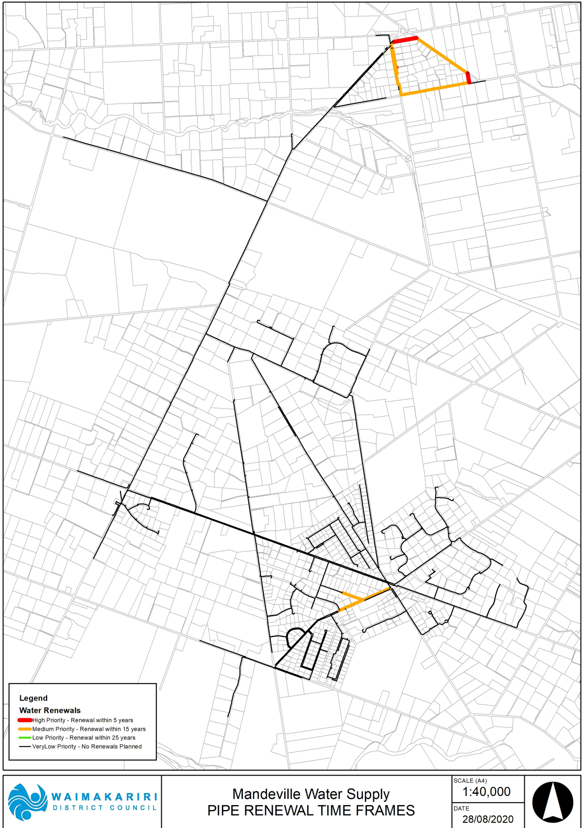
Figure 8: Pipe Renewal Time Frames
