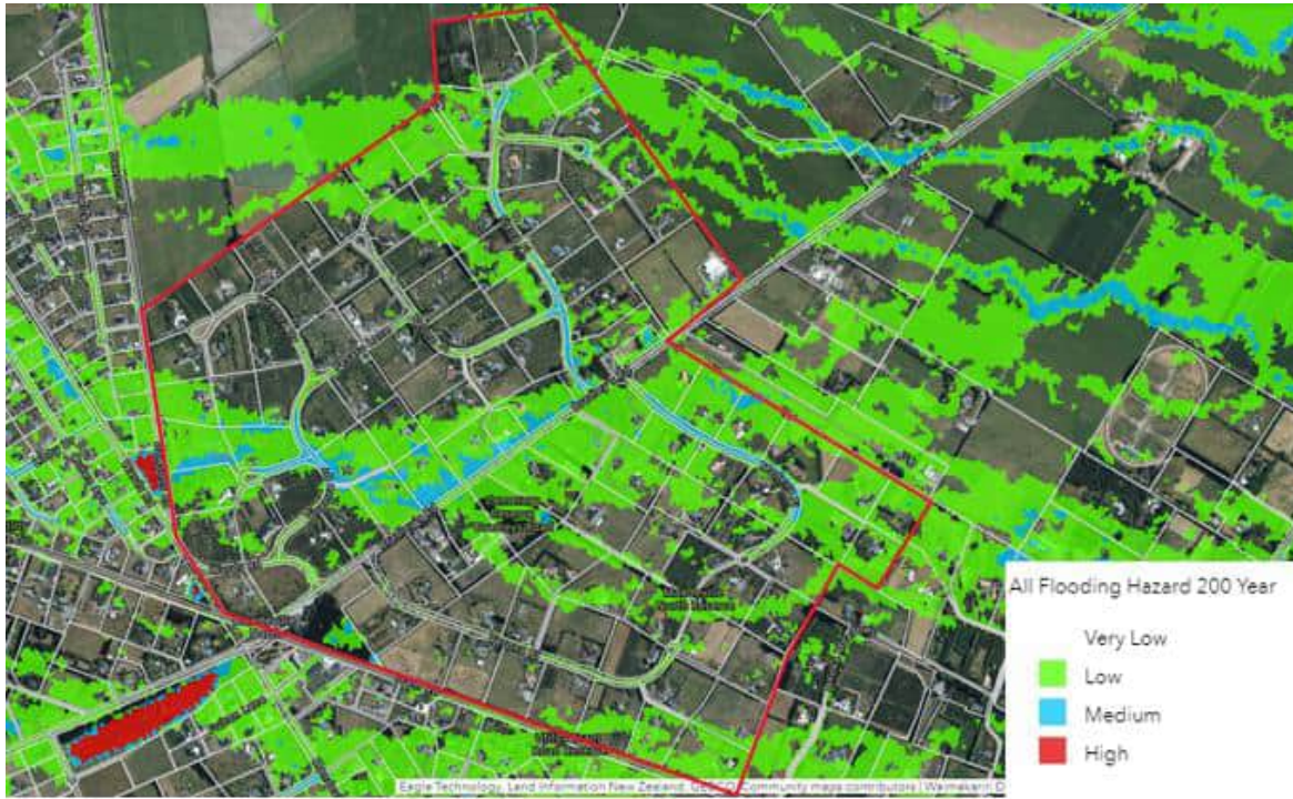
Figure 4. Current Level of Flood Hazard at the Site (source: Waimakariri Flood Hazard Map)
