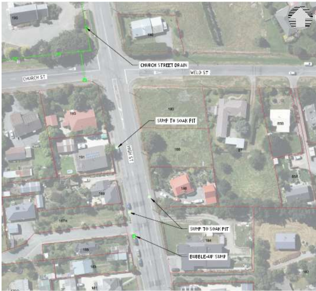
Figure 2: Existing Drainage - 189 High Street
