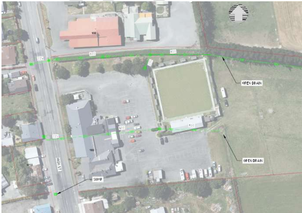
Figure 3: Existing Drainage - Oxford Working Mens Club, High Street
