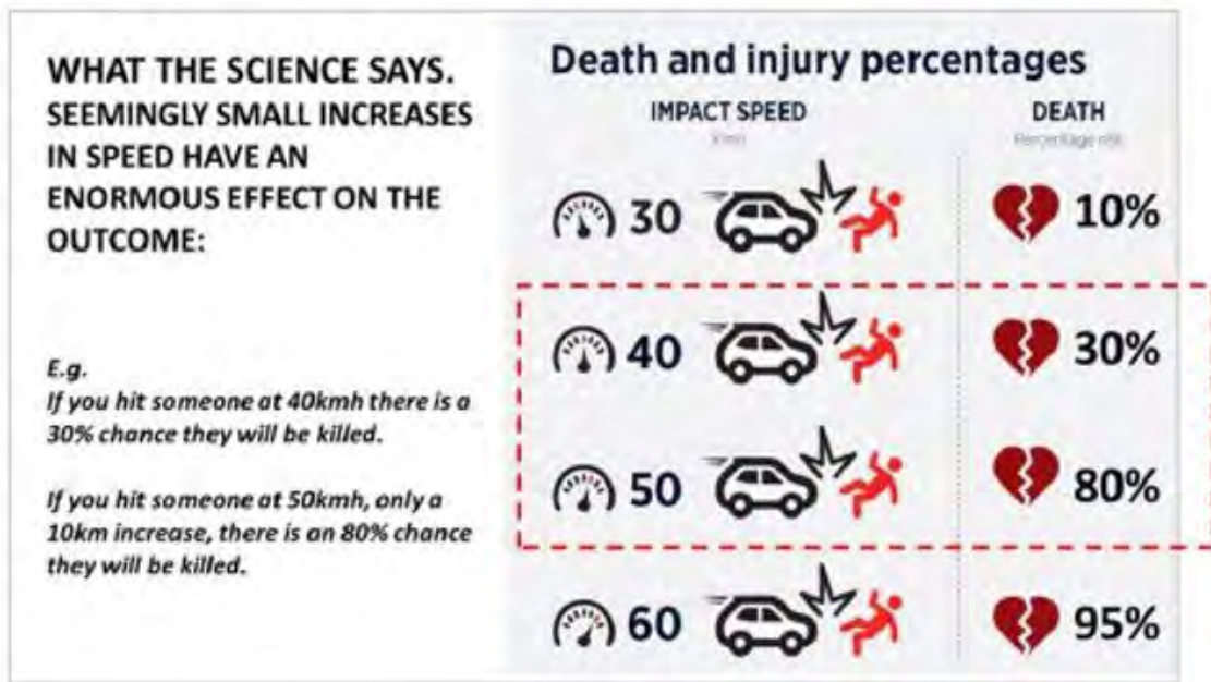
Figure 3. Likelihood of death for pedestrians hit at different vehicle speeds (Auckland Transport, 2022).
