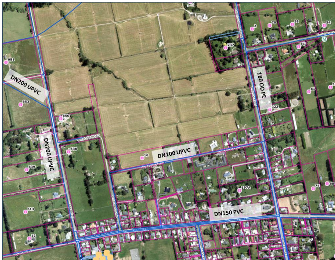
Figure 9. Existing Water Supply Network
