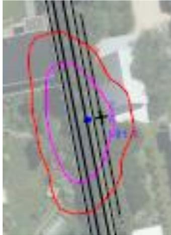
To overcome this issue, the pole mounted luminaires within this section should be swapped out for dark-sky compliant bollard lights. These require installation at closer spacing, but do not adversely impact the neighbouring properties.
