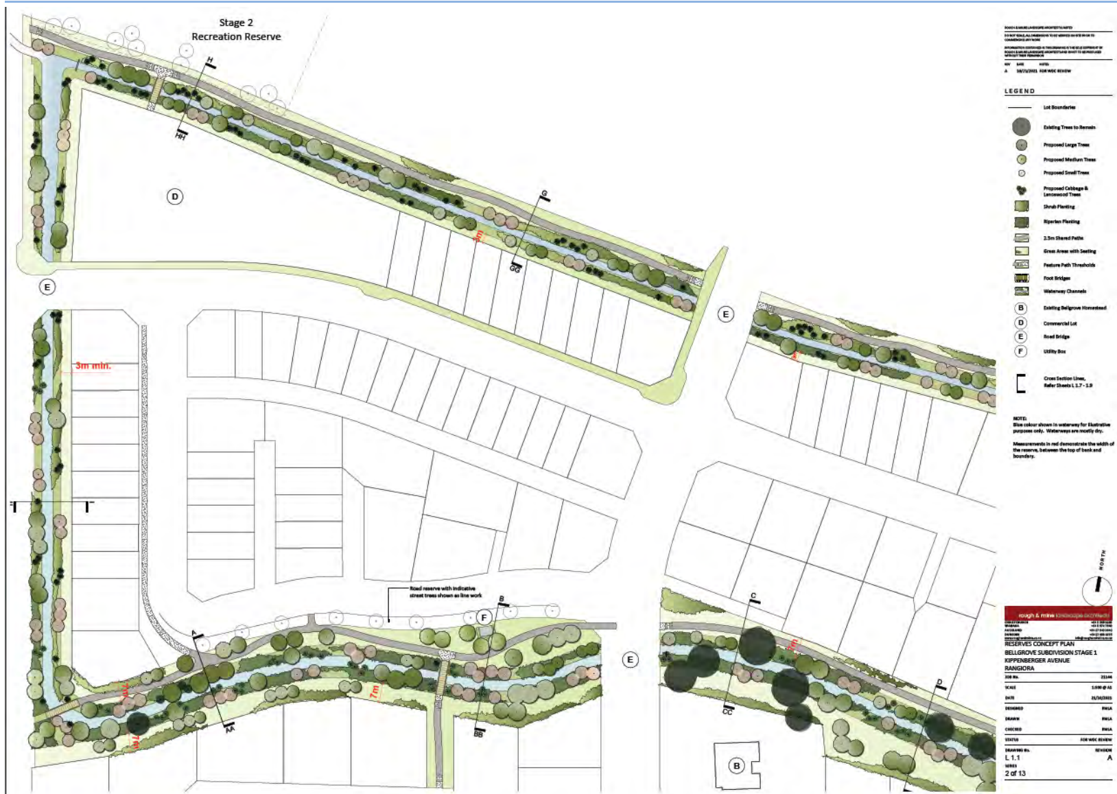
Figure ii. Proposed minimum setback widths (7 m plus vegetated buffer) in the October landscape plans for the Cam / Ruataniwha River.
