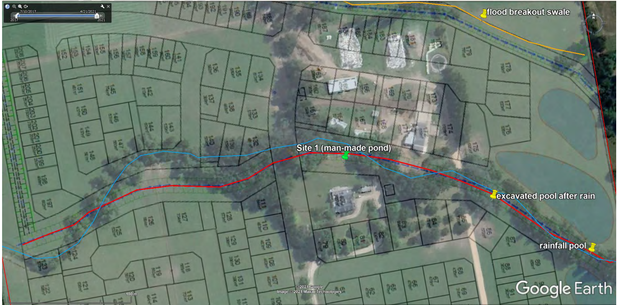
Figure i. Proposed re-alignment of the Cam / Ruataniwha River headwaters (red line), with existing course (blue line). The lot numbers are old and have been superseded.
