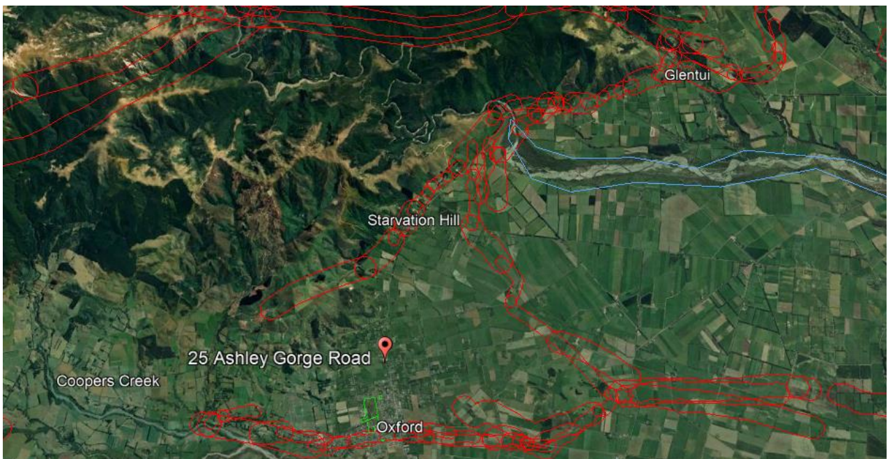
Figure 2: Updated active fault information from Canterbury Maps Fault Awareness Areas (2019).
