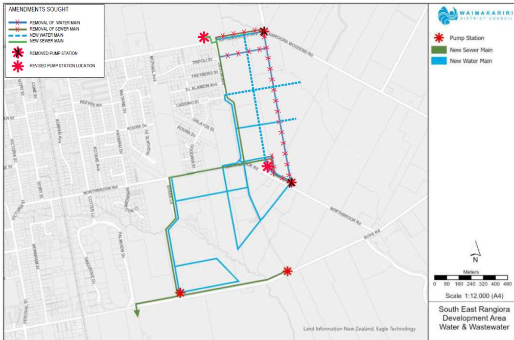
Figure 2B-5. Changes Sought by Bellgrove to the SER ODP - Water and Wastewater Layer
