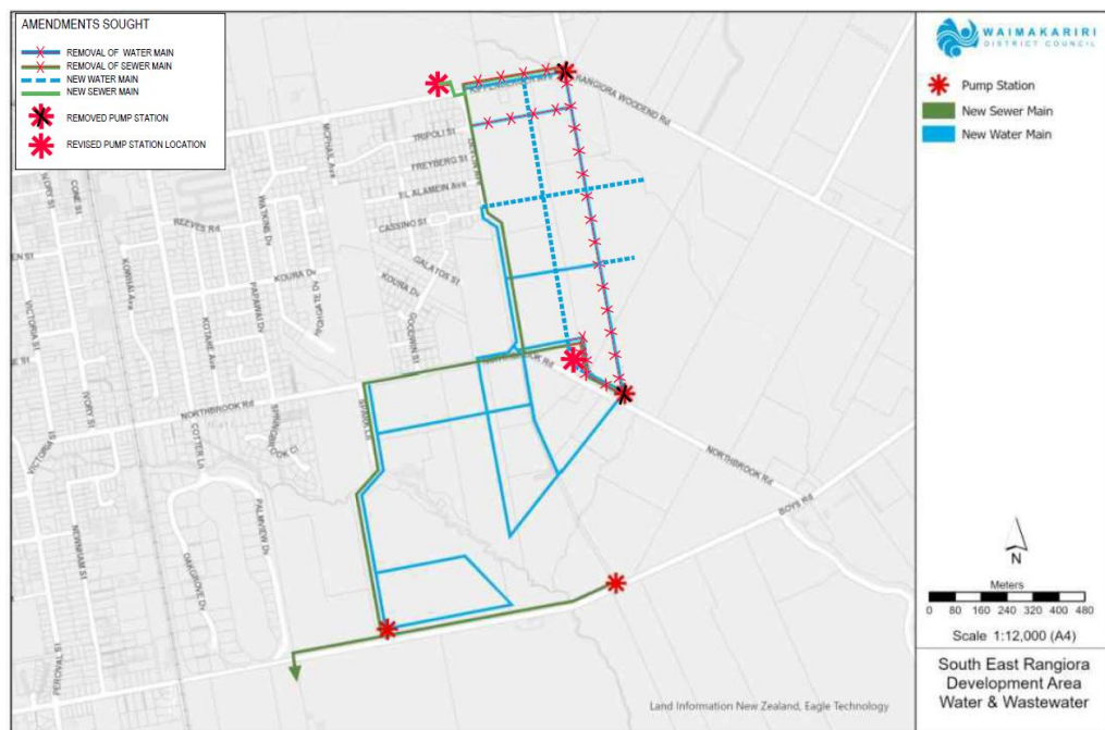
Figure 4. Changes Sought by Bellgrove to the SER ODP – Water and Wastewater Layer
