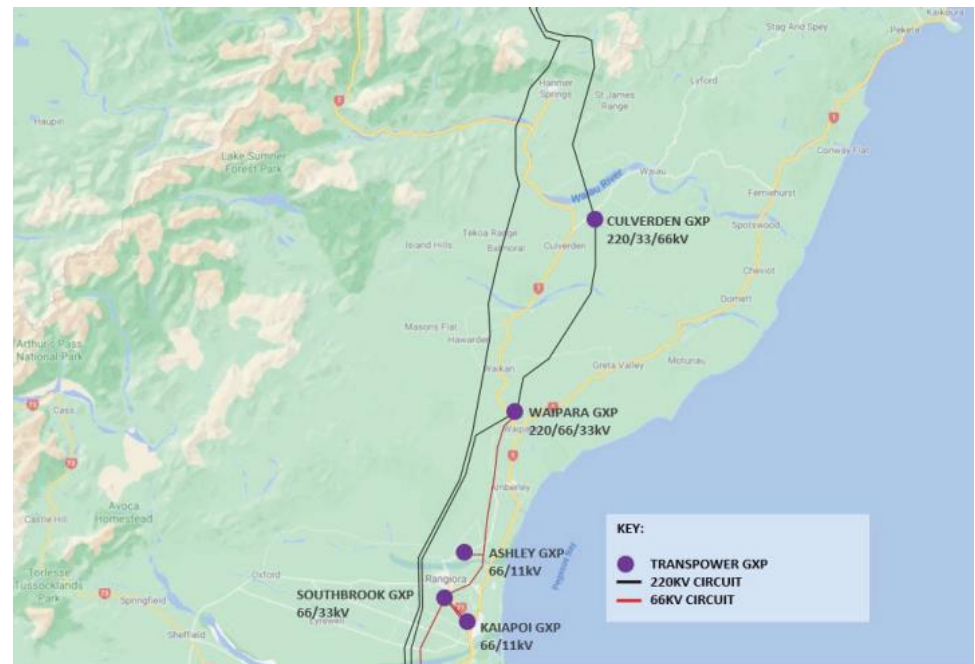
Figure 2: MainPower's North Canterbury Transmission Grid
