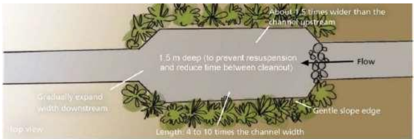
Figure 13: Sediment Trap Design
