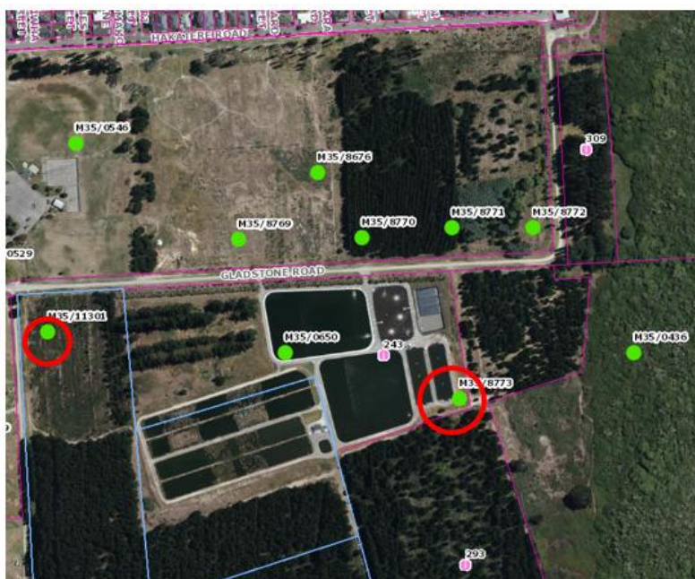
Figure 34: Location of south-east down-gradient (M35/8773) and south-west up-gradient (M35/11301) groundwater monitoring bores
