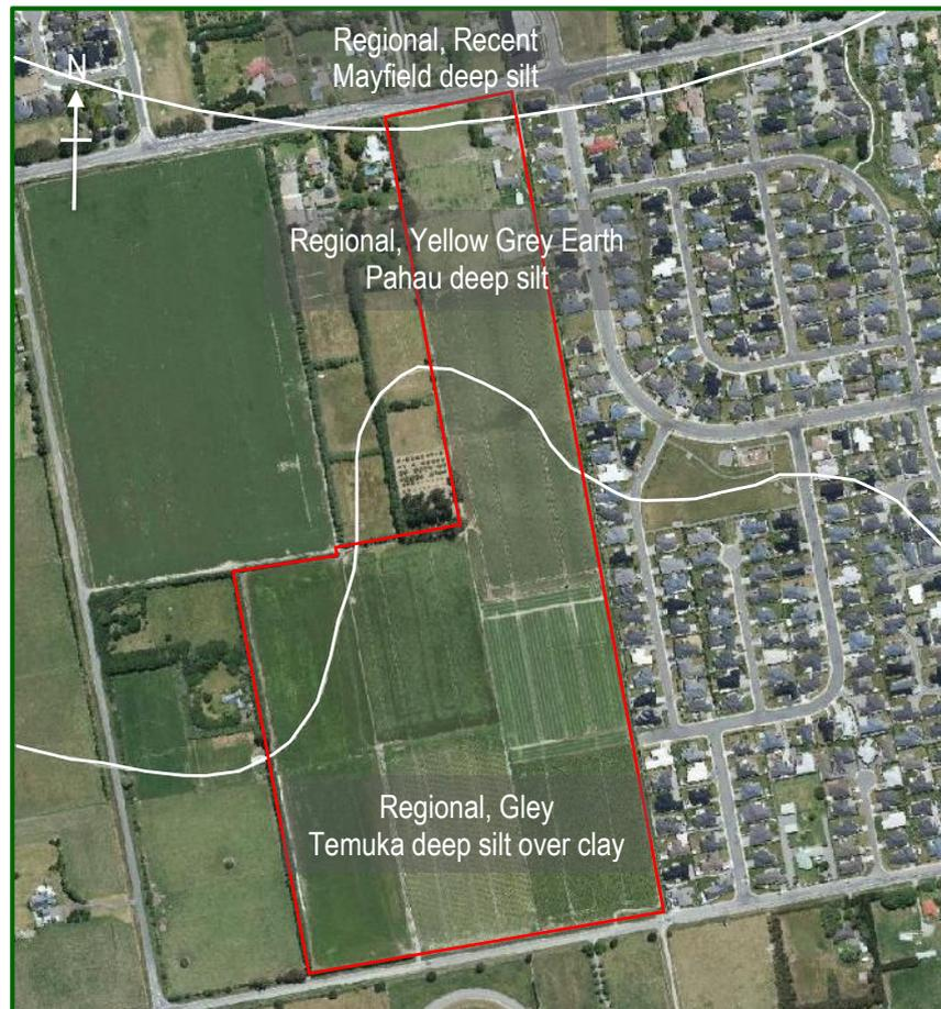
Figure 2 – Soil Type Plan
