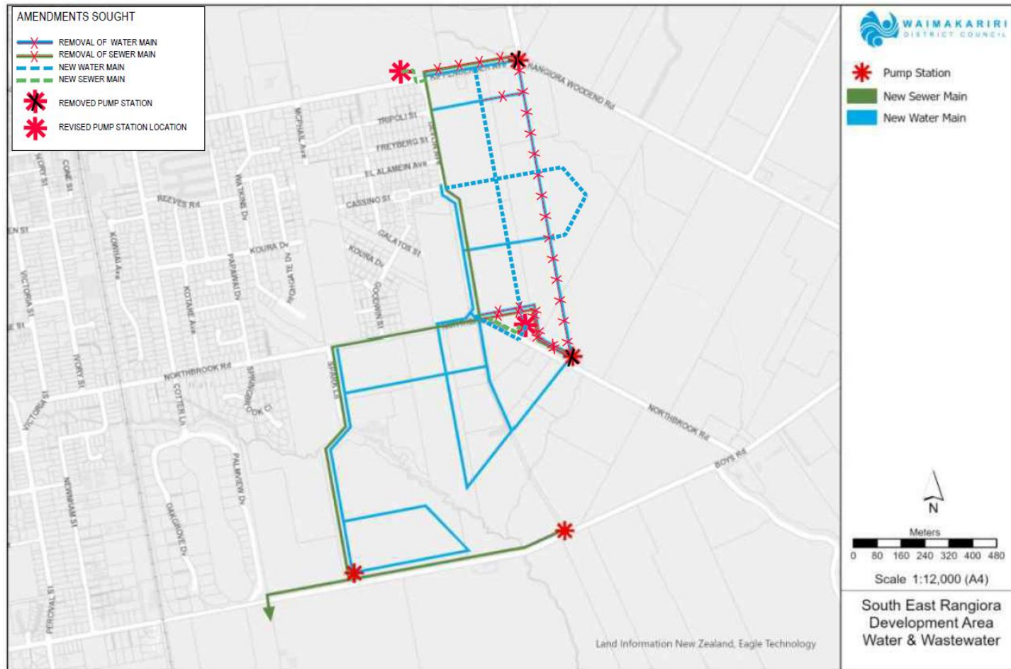
Figure 2B-2. Revised Water and Wastewater SER-ODP
