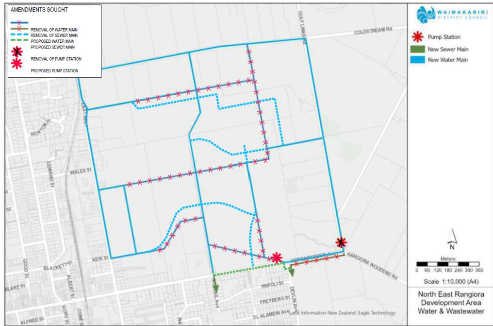
Figure 3C-5. Bellgrove Changes Sought to the North East Rangiora Water and Wastewater Outline Development Plan Option B
